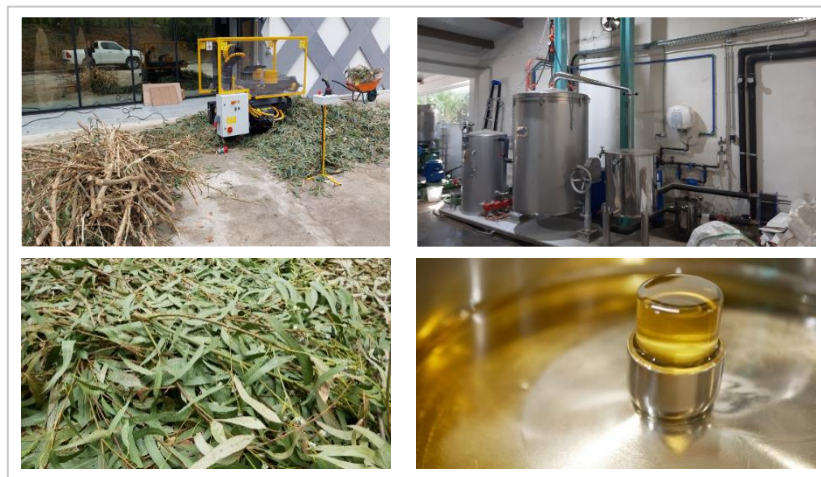
Figure 6 – Preparation of biomass, pilot unit for steam distillation and essential oil produced
