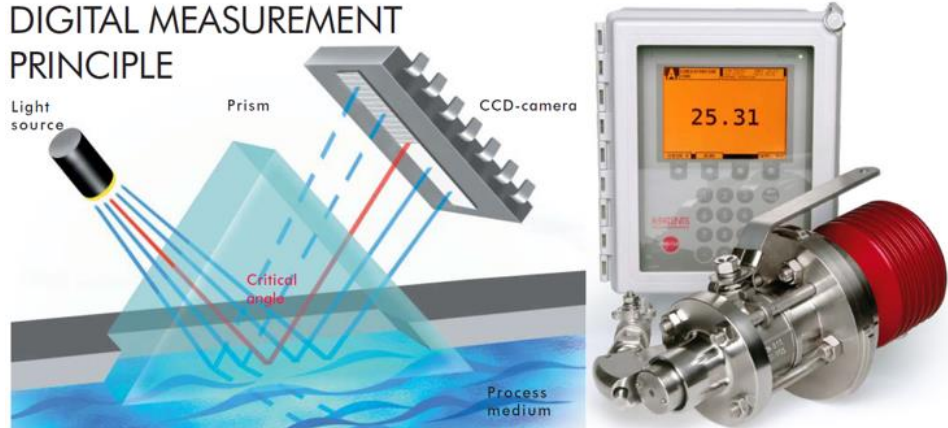
Figure 1. Refractive index digital measurement principle and sensor.
