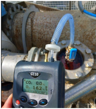
Figure 5. Sampling point and measurement for the residual gas in the reactor two.
