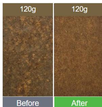
Figure 5. Formation before and after Sleeve roll installation
